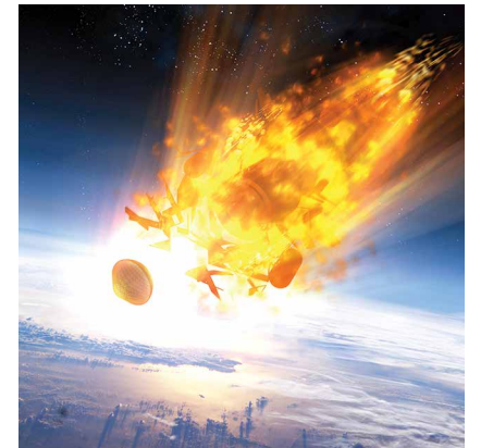
In this visualization, a reentry black box data recorder survives destruction of its host spacecraft during atmospheric breakup, improving orbital debris hazard prediction and reentry safety knowledge.
